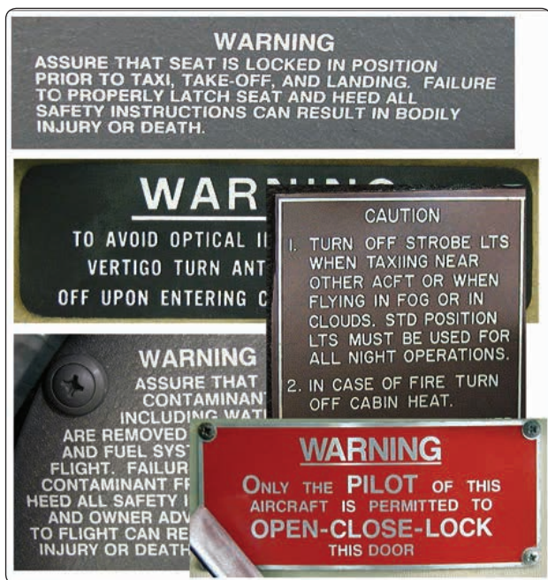
Figure 9-5. Placards are used to depict aircraft limitations.
