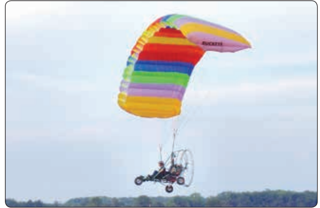
Figure 5-20. A powered parachute.
