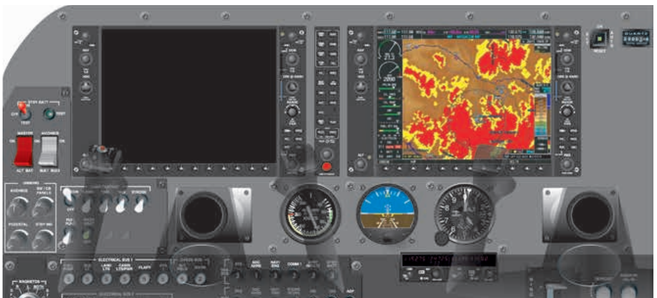
Figure 8-13. Multi-function display (MFD).
