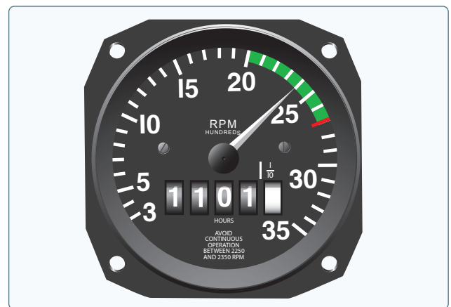
Figure 7-8. Engine rpm is indicated on the tachometer.
