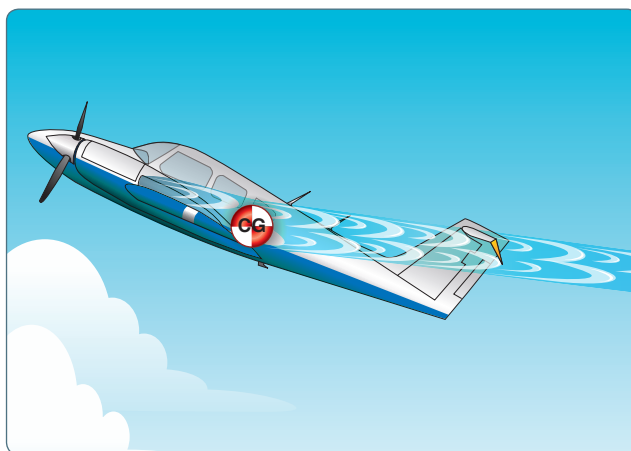
Figure 6-11. Aircraft with a T-tail design at a high AOA and an aft CG.
