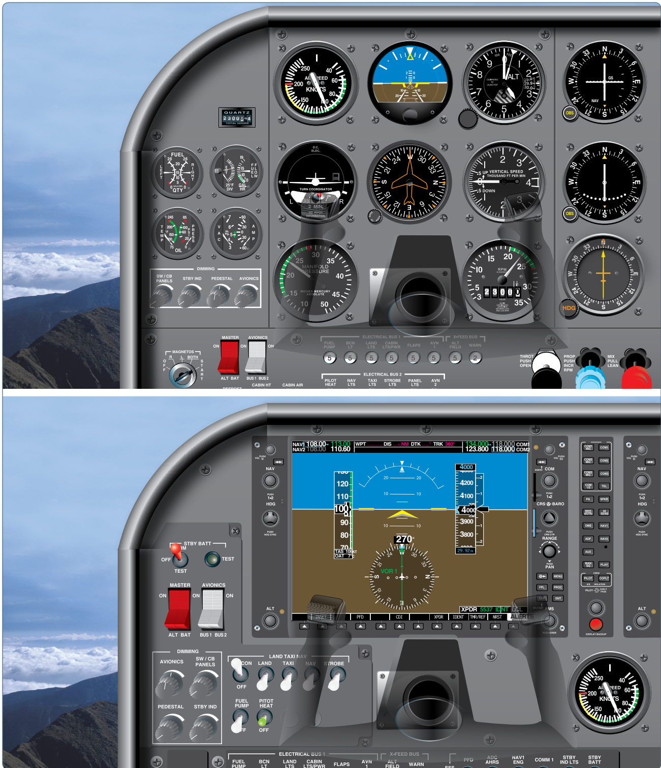
Figure 2-22. Two similar flight decks equipped with the same information two different ways, analog and digital. What are they indicating? Chances are that the analog pilot will review the top display before the bottom display. Conversely, the digitally trained pilot will review the instrument panel on the bottom first.
