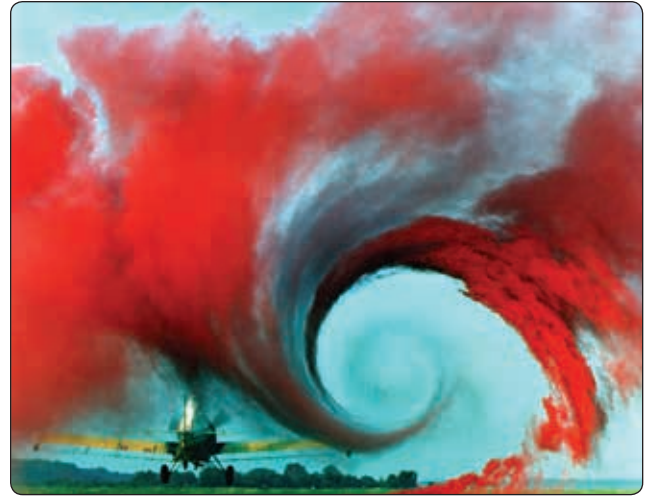
Figure 5-9. Wingtip vortex from a crop duster.
